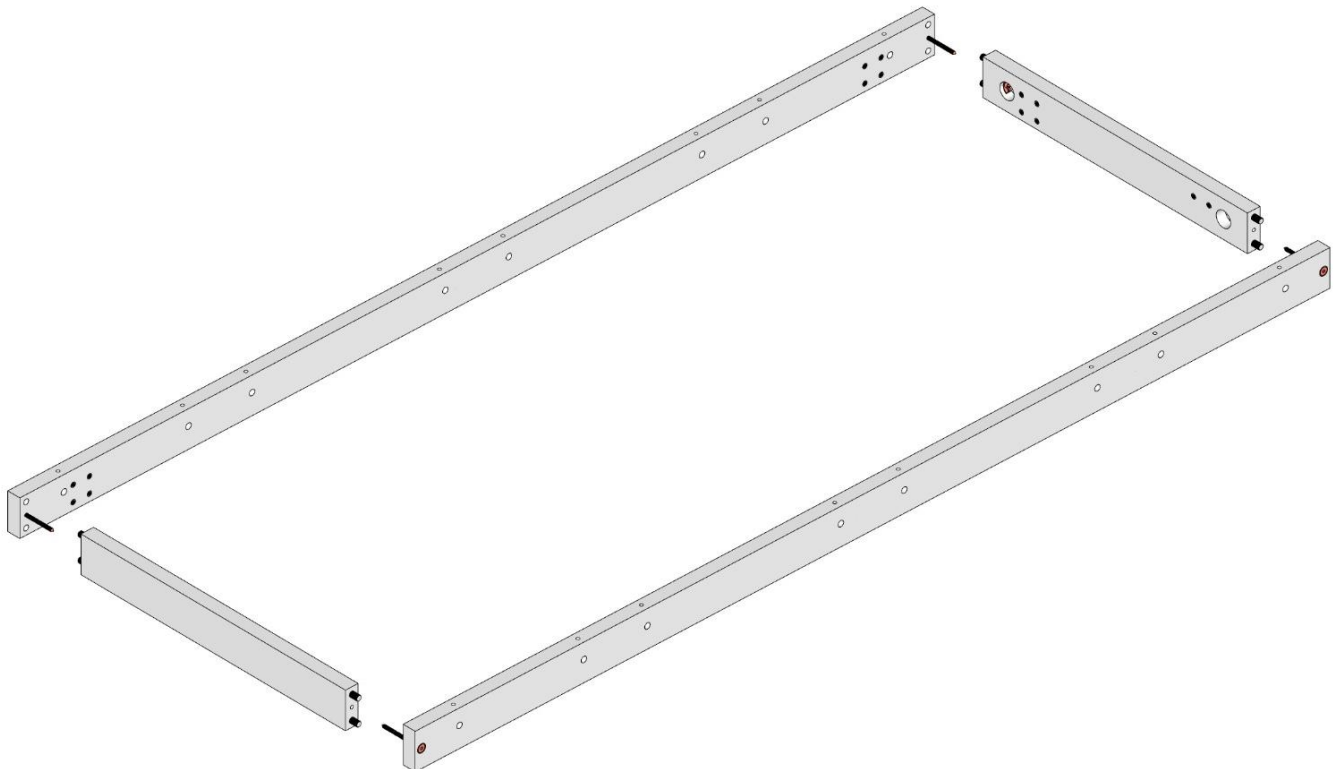
Rail layout before joining the four corners
